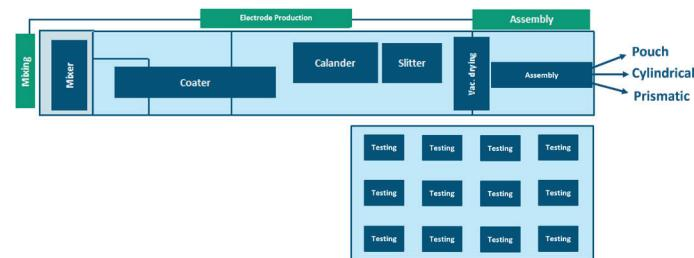
*From powder to cell: The pilot line covers the complete process chain — from electrode production to final cells in three different formats (pouch, cylindrical, prismatic).*
