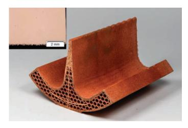
Fraunhofer USA is collaborating with Fraunhofer IWS to evaluate the use of these new laser technologies for additive manufacturing of copper components. Fraunhofer IWS is focusing on Laser Powder Bed Fusion technology (L-PBF), whereas Fraunhofer USA CMW is focusing on Laser Direct Energy Deposition technology (L-DED).
