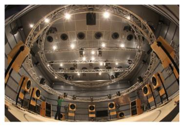
HE-AAC and other audio codecs are developed and tested in Fraunhofer's advanced sound lab that allows for critical listening and flexible loud speaker arrangement.
