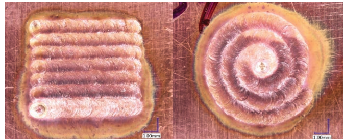
© Fraunhofer USA, Examples of weld patterns generated using K-Lab Scout Vision System and single-mode IR laser
