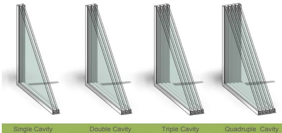
Figure 4. Inserts with several Low-E foils to further reduce thermal energy losses
