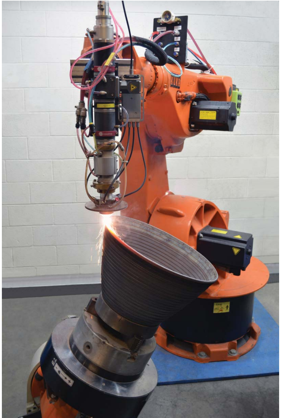
Laser Additive Manufacturing of Nozzle Demonstration Component at CLA
