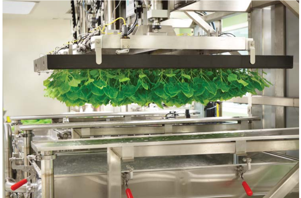
Tray of Nicotiana benthamiana plants about to be placed in vacuum infiltration chamber
